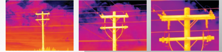
Standard (left), 2x telephoto (center) and 4x telephoto (right)—see the right level of critical infrared detail
